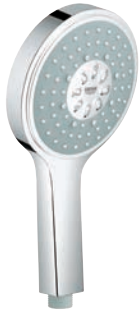
27 664 000 / 27 663 LSO Hand shower 130 4+ spray patterns: GROHE Rain O 2 , Rain, Bokoma Spray, Jet with 9.5 l/min. GROHE EcoJoy
